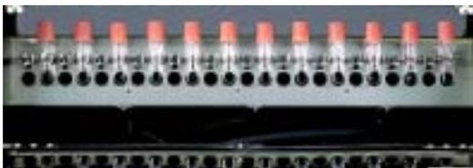
A temperature gradient can be applied to 2 rows of 24 samples in culture tubes between 5 and 70°C. Tubes are easy to insert and remove yet are held tightly in place along the incubator block.
